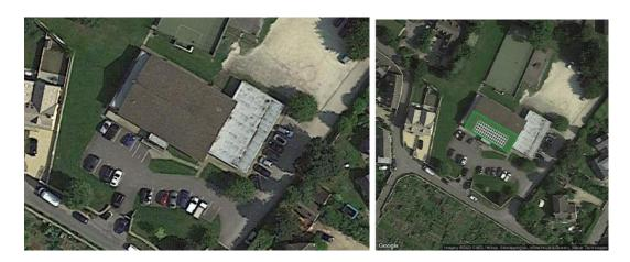
As the overhead views of the Hub above show, the Hub has a pitched roof area facing roughly south-west. The image on the right shows the proposed layout of the 60 PV panels required. The panels will be installed such that they comply with Permitted Development criteria for roof – mounted PV. As the Hub is not within the Minchinhampton Conservation Area, it does not require planning permission.
